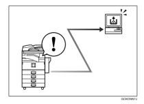
You can monitor machine status and change settings using a computer.
